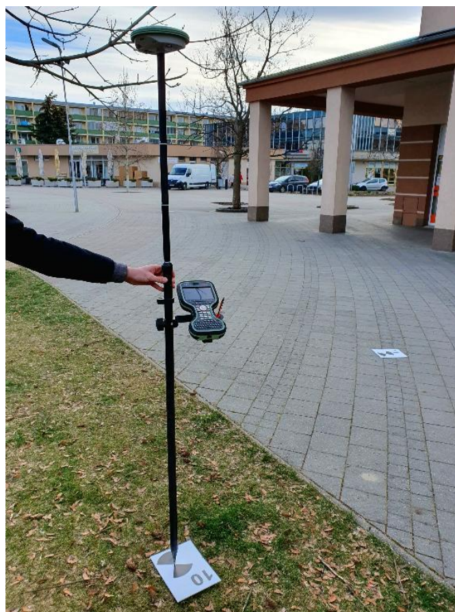
Fig. 2. GNSS set Leica GS07 Source: Own elaboration
