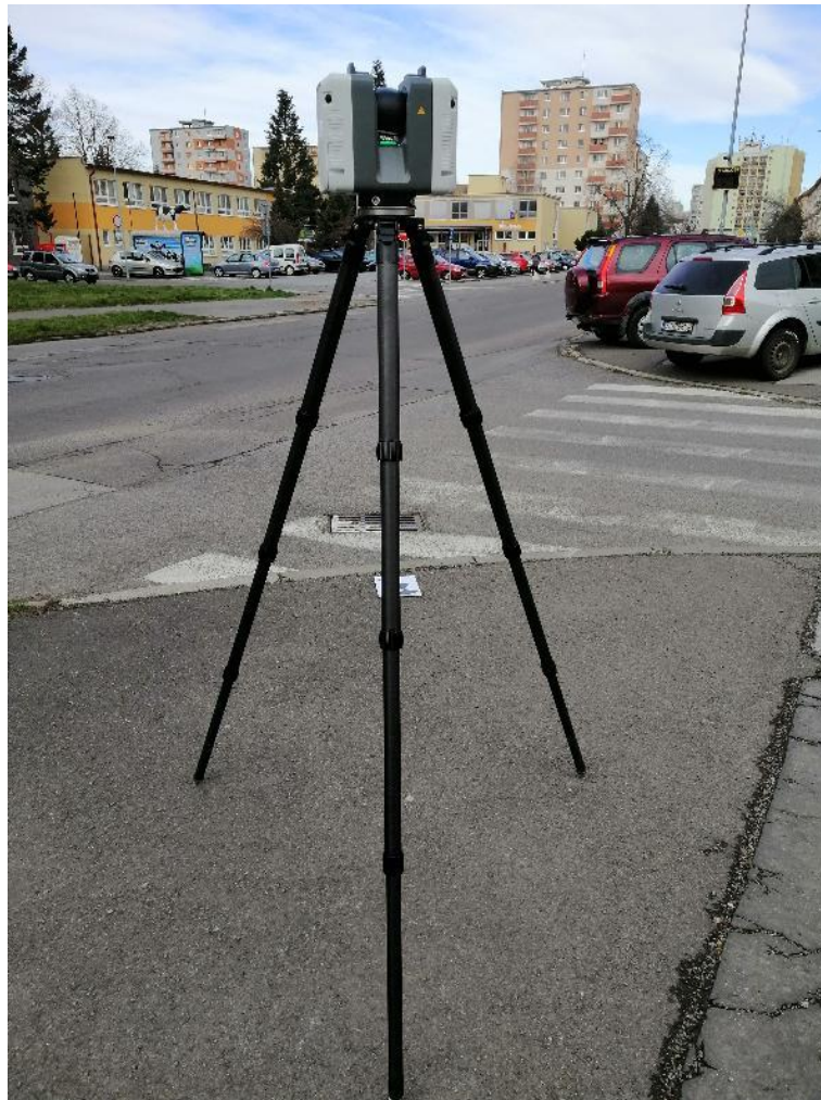
Fig. 3. Terrestrial laser scanner Leica RTC 360 Source: Own elaboration
