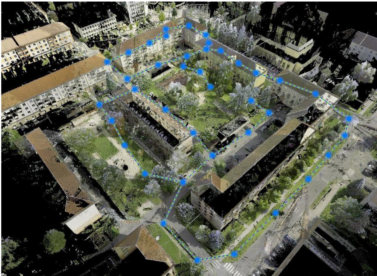
Fig. 5. Distribution of setups in surveying by TLS method Source: Own elaboration
