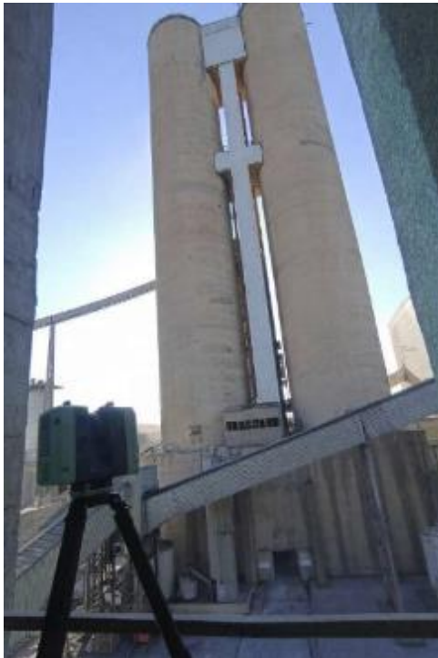
Fig. 3. Scan positions of TLS during the scanning of the homogenization silos Source: own elaboration
