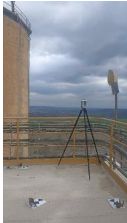
Fig. 3. Scan positions of TLS during the scanning of the homogenization silos Source: own elaboration
