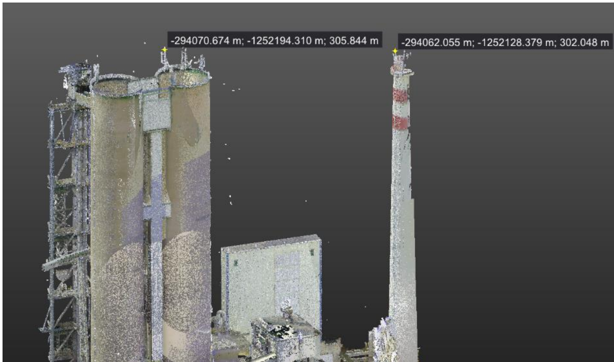
Fig. 9. Height determination from TLS point cloud Source: own elaboration
